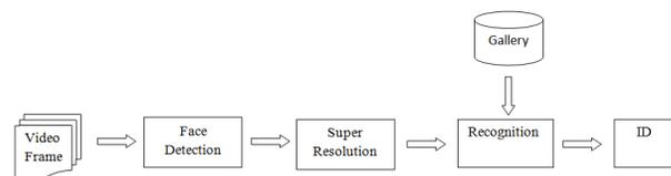
Fig. 1. Flow chart of FR using super-resolution reconstruction from low resolution (LR) images.
