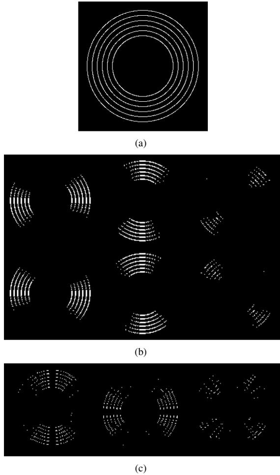
Fig. 4. Binary image (256x256) depicting circles with different radii. (a) Synthetically generated circles with different radii. (b) Output of 2D DTCWT. One can observe that each wavelet subband responds for particular orientation, and 2D DTCWT can discriminate between positive and negative orientations. (c) Output of ordinary DWT. One can observe that DWT can not distinguish orientations  $-45^\circ$  and  $45^\circ$ .
