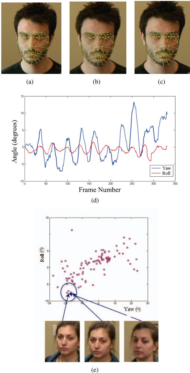
Fig. 2. Output of ASM for (a)  $-8^\circ$ , (b)  $0^\circ$ , (c)  $-16^\circ$  respectively. Poses are estimated using the PittPatt SDK [18]. (d) Pose estimated by PittPatt SDK. The line in blue shows the variation of yaw, while the red line shows the variation of roll across time. Notice that the changes are periodic over time. (e) By plotting yaw vs roll we can find the nearest neighbors to form a group of similar poses for reconstruction of a super-resolved image.
