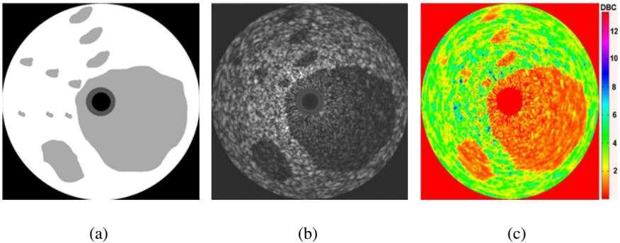
**Fig. 1.** (a) Mask used for creating the synthetic IVUS data, (b) its corresponding IVUS B-mode reconstruction, and (c) recovered DBC values using 100 samplings ( $\Delta P = 0.05 \text{ mm}$ ,  $\beta = 1$ , and  $\delta = 3$ )
