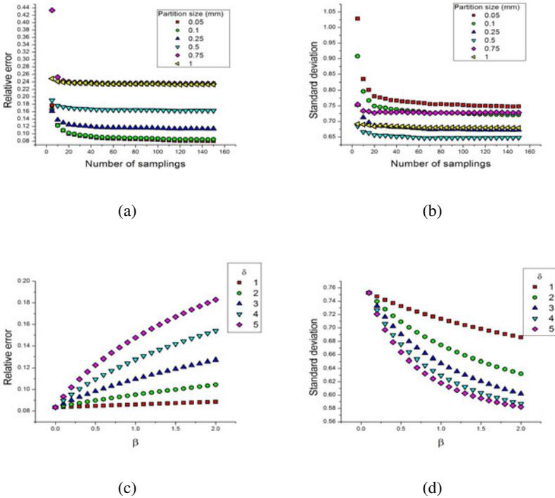
**Fig. 2.** (a, c) Relative error and (b, d) standard deviation for the mean of the recovered DBC values for two type of scatterers with respect to (a) the size of partition and (b) number of samplings, and (c) the cardinality of neighbors and (d) the value of the regularization term
